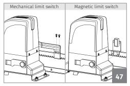
$\mathbf{02}$  • Put the DIN912 M5 x 12 screws supplied with the accessories until the limit-switch plate is fixed to the rack.
