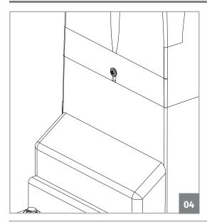
During installation you will need to open the motor cover, to access various components on the inside. For this, loosen the 2 screws identified with (A) until the cover is free to be removed.
