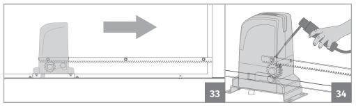
**04** • Close the gate a bit until the other end of the rack rests on top of the pinion and weld the other spacer to the gate.
