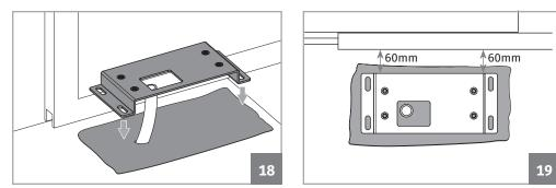
**01** • Place the fixing plate on top of the foundation and align it parallel to the gate, keeping a distance of 60mm between them, as visible in Figure 19.
