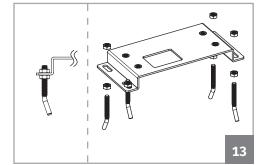
**02** • Fill the hole with fresh concrete and smooth the top part where you will fix the plate.
