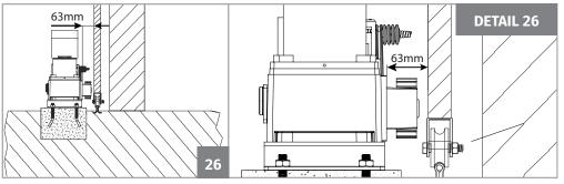
**03** • Align it parallel to the gate leaving a distance of 63mm between them, as visible in the image 26. Oval holes of the motor should be centered with the threaded holes in the fixing plate, as visible on DETAIL 26.
