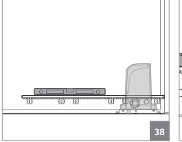
01 • Place a piece of rack on top of the pinion and level it horizontally with a level.
