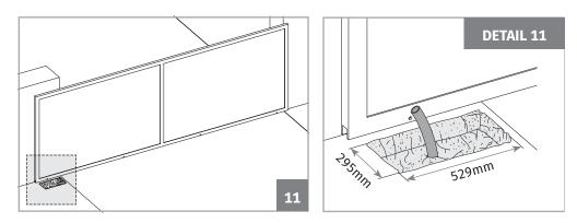
**01** • Make a hole in the ground to create a foundation in concrete. The dimensions shown are these recommended to create the foundation. You must leave tubes in the middle of the hole for the passage of cables for power and accessories, as shown in the detail of image 11.
