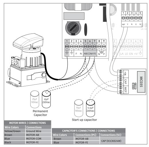
The motor connections must be made as shown above, by connecting the 4 motor wires to the appropriate inputs of the control board.
