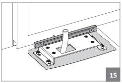
**04** • Insert the plate with screws in the concrete while it is still fresh and level it horizontally with a level. Also align it parallel to the gate, keeping a distance of 60mm between them, as visible in picture 16.
