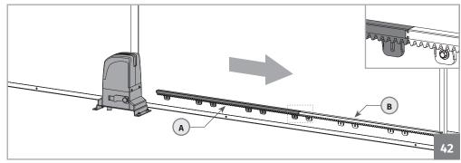
**04** • Close the gate a bit, so that the rack is not being supported on the pinion anymore and apply another piece of rack (**A**), fitting it into the rack already installed (**B**), as you can see in detail of image 41.
