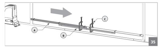
**05** • Close the gate a bit, so that the rack is not being supported on the pinion anymore and apply another piece of rack (A). To synchronize the teeth with the piece already installed, use an additional piece of rack (B) and place it under the union of the other two, holding them with clamps (C).
