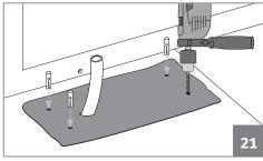
**03** • Drill four holes with Ø18mm on foundation. Place M10 steel anchors on the holes.
