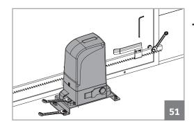
Check all screws of the automation such as the fixing plate to the ground, the plates of the limit switches, motor and the gear rack.
