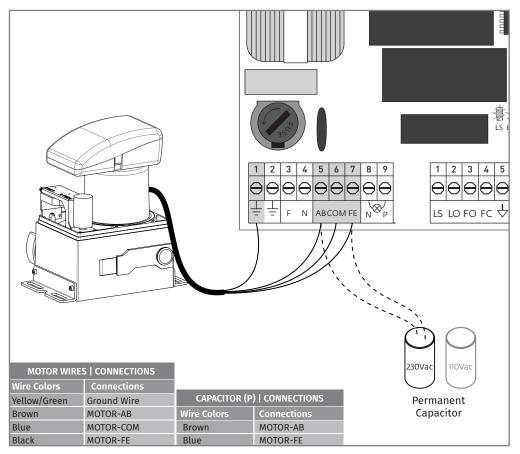
The motor connections must be made as shown above, by connecting the 4 motor wires to the appropriate inputs of the control board.
