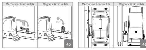
**01** • Place the opening limit-switch plate in the rack so that it can trigger the limit-switch of the motor before the gate gets to opening stopper. The mechanical limit switch is activated when the plate is in contact with the spring. The magnetic limit switch is activated when the magnet is aligned with the motor reader (Fig. 45).
