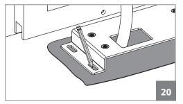
**02** • Mark the place to make the holes for the bushings. Must make the mark at the center of the oval holes of the plate.
