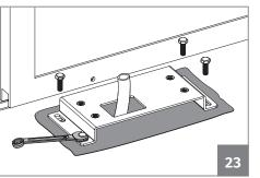
**04** • Place the fixing plate on the foundation in cement respecting the distances of image 19. Use a level to levelit horizontally and fasten it with M10 screws.
